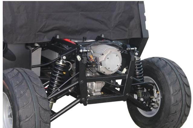
**Front differential** - Featuring Electric Differential Lock System. Simply push the button on the dash control that is exposed when the vehicle is in 4WD mode and the front differential locks so that both front wheels are in drive mode.
